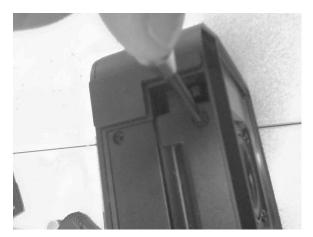
3. USE A TORX HEAD (size T-6) SCREWDRIVER TO REMOVE 6 SCREWS
