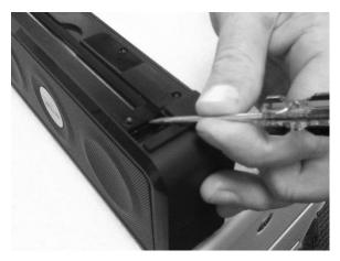
4. USE FLATHEAD SCREWDRIVER TO PRY LID FROM HOUSING. THE DOOR IS AFFIXED TO THE HOUSING WITH ADHESIVE TAPE.
