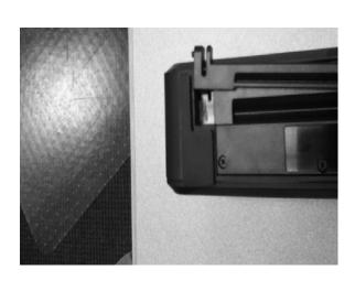
1. USE FLATHEAD SCREWDRIVER TO PRY KICKSTAND ATTACHMENT LEG FROM HOLE
