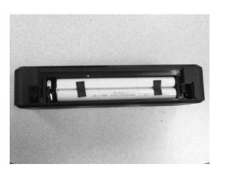
8. REPLACE WITH NEW BATTERY AND PLUG BATTERY CONNECTOR WITH HOUSING CONNECTOR
