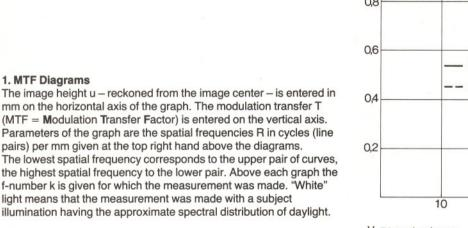
Unless otherwise indicated, the performance data refer to large object distances, for which normal photographic lenses are primarily used.
